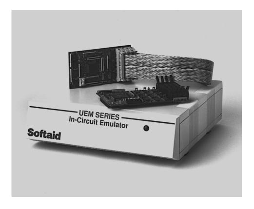
The built-in performance analyzer tracks execution time of up to 255 functions simultaneously, in real time.
